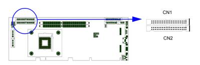
You can attach up to four IDE (Integrated Drive Electronics) drives to the PCA-6186's built-in controller. The primary (CN1) and secondary (CN2) connectors can each accommodate two drives.
